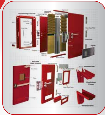
Steel Door Construction Overview
